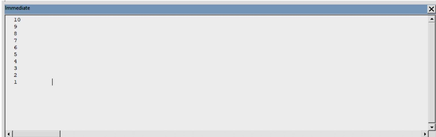
The screenshot shows the Immediate window in VBA, which displays the output of the program. The output consists of the numbers 10, 9, 8, 7, 6, 5, 4, 3, 2, and 1, each on a new line. The window has a title bar that says "Immediate" and a close button (X) in the top right corner. There are also scroll bars on the right and bottom of the window.
