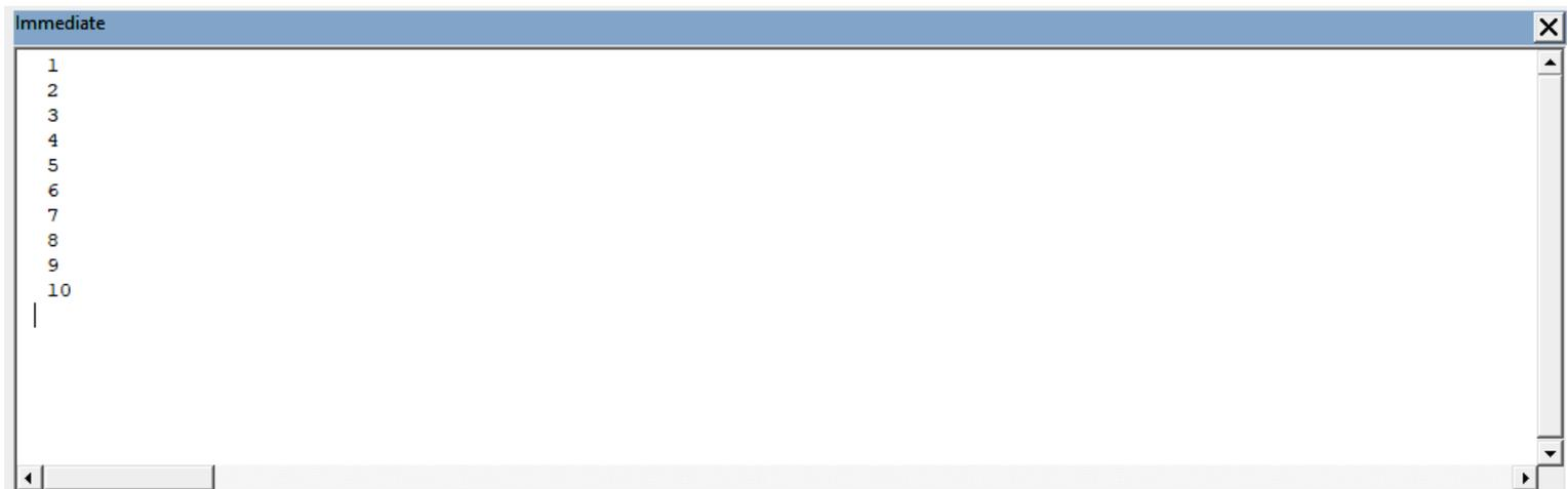
The screenshot shows the Immediate window in VBA, which displays the output of the program. The output consists of the numbers 1 through 10, each on a new line, indicating that the loop executed successfully and printed each number in sequence.
